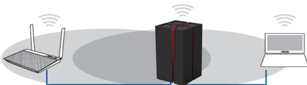
The ideal location for RP-AC68U is between your wireless router and wireless device.
