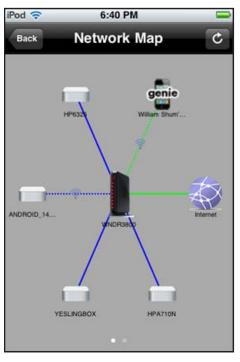
You can use the C Refresh button to update the screen at any time. A good connection is shown in green. A red line indicates a connection that is not working.
