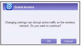
This message reminds you that changing the wireless settings will disconnect any computers or devices that are currently connected wirelessly to the network.
