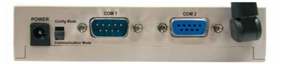
**POWER** Plug in the power adapter of 12V DC/1A into the power port.
