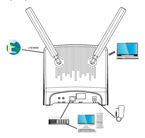
**Step 1** Connect the supplied power adapter to the CPE.
