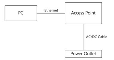
**Note**: ERA150 supports both IEEE 802.3af PoE (Power over Ethernet) and regular power adapter. You should use either one as the power source. Please do not apply both at the same time.
