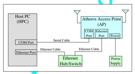
Figure 1 – Connection Between AP and Host PC
