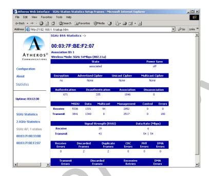
Figure A-16. Basic Service Set Statistics Window for Station
