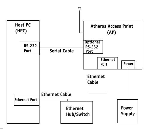
Figure 2-1. Access Point to HPC Connections
