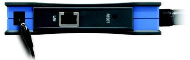
Figure 4-2: Connect the Power
