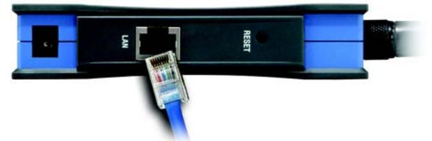
Figure 4-1: Connect to the Network
