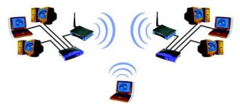
Figure 2-3: Network Using Wireless Bridging
