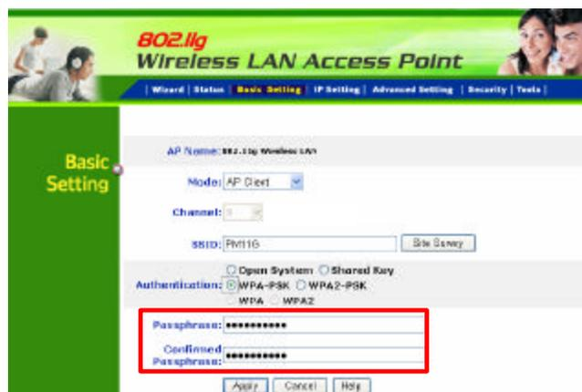
**Apply:** For the changes made to any of the items above to be effective, click “Apply”. The new settings are now been saved to Access Point and will be effective once the Access Point restarts.
