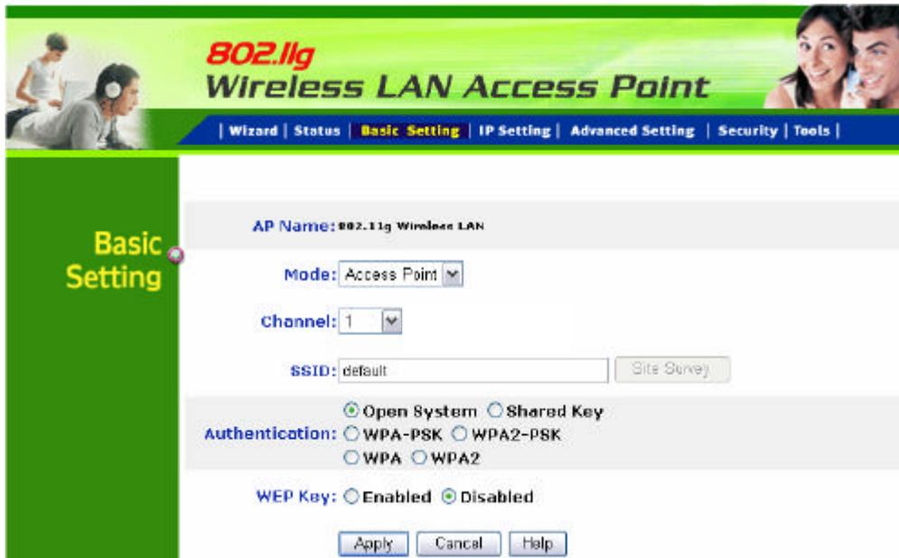
The screenshot shows the configuration interface for an 802.11g Wireless LAN Access Point. The page title is "802.11g Wireless LAN Access Point" and the current tab is "Basic Setting". The configuration options are as follows:
