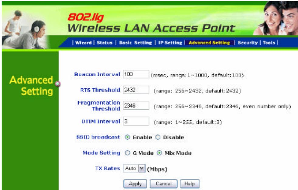
The screenshot displays the 'Advanced Setting' page for an 802.11g Wireless LAN Access Point. The page features a navigation bar with links for Wizard, Status, Basic Setting, IP Setting, Advanced Setting (highlighted), Security, and Tools. A green sidebar on the left contains the text 'Advanced Setting'. The main content area includes the following settings:
