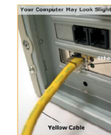
**Step 2** Repeat these steps for each computer that you want to connect to the FiOS Router using Ethernet.
