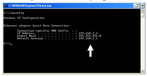
NOTE: If the IP address of Gateway is not displayed, or the address followed by 'IP Address' begins with '169', please recheck network connection between your computer and router, and / or go to the beginning of this chapter, to recheck every step of network setup procedure.
