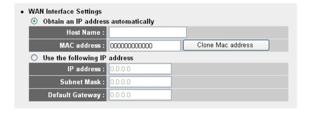
Please select the type of how you obtain IP address from your service provider here. You can choose 'Obtain an IP address automatically' (equal to DHCP, please refer to 'Cable Modem' section above), or 'Use the following IP address' (equal to static IP address, please refer to 'PPPoE xDSL' section above).
