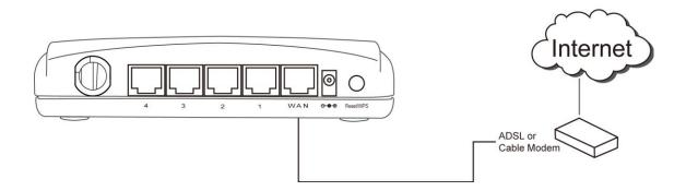
2. Connect all your computers, network devices (network-enabled consumer devices other than computers, like game console, or switch / hub) to the LAN port of the router.
