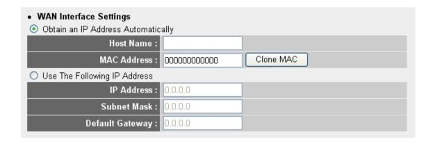
Select the type of how you obtain IP address from your service provider here. You can choose 'Obtain an IP address automatically' (equal to DHCP, please refer to 'Cable Modem' section above), or 'Use the following IP address' (i.e. static IP address)
