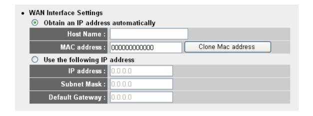
Please select the type of how you obtain IP address from your service provider here. You can choose 'Obtain an IP address automatically' (equal to DHCP, please refer to 'Cable Modem' section above), or 'Use the following IP address' (equal to static IP address, please refer to 'PPPoE
