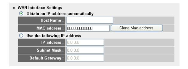
Select the type of how you obtain IP address from your service provider here. You can choose 'Obtain an IP address automatically' (equal to DHCP, please refer to 'Cable Modem' section above), or 'Use the following IP address' (i.e. static IP address)
