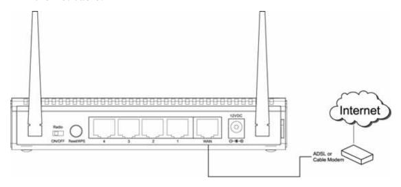
2. Connect all your computers, network devices (network-enabled consumer devices other than computers, like game console, or switch / hub) to the LAN port of the router.
