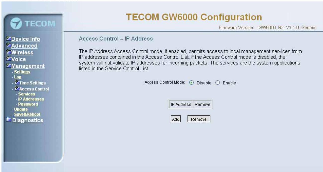
Figure 6-47-1. Management – Access Control – IP Addresses
