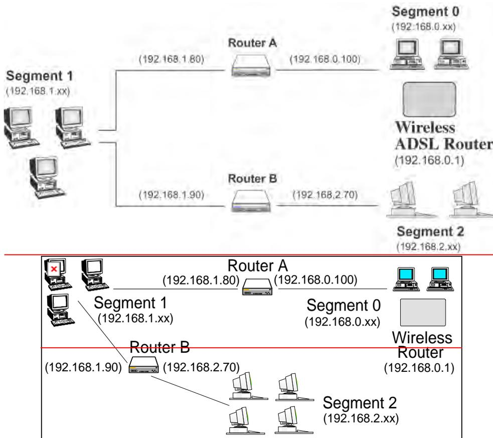
Figure 69: Routing Example
