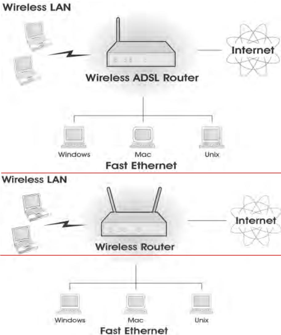
Figure 1: Wireless ADSL Router
