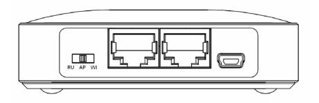
Note: 1. Before sliding the switch modes, please power-off the router firstly. Moreover, please stay over 10 seconds between power-off / power-on condition.
