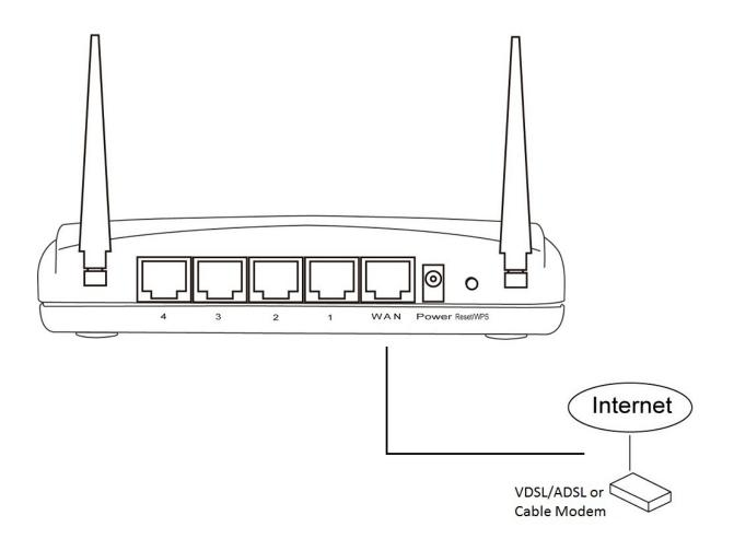
Connect all your computers, network devices (network-enabled consumer devices other than computers, like Game console, or Switch / Hub) to the LAN port of the router.
