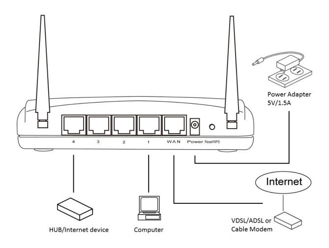
4. Please check all LEDs on the front panel. 'PWR' LED should be steadily on, WAN and LAN LEDs should be on if the computer / network device connected to the respective port of the router is powered on and correctly connected. If PWD LED is not on, or any LED you expected is not on, please recheck the cabling, or jump to '4-2 Troubleshooting' for possible reasons and solution.
