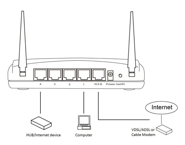
3. Connect the power adapter to the wall outlet, and then connect it to the 'Power jack' of the router.
