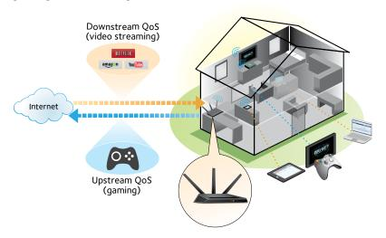
To set up QoS, log in to the router and enable Downstream QoS and Upstream QoS.
