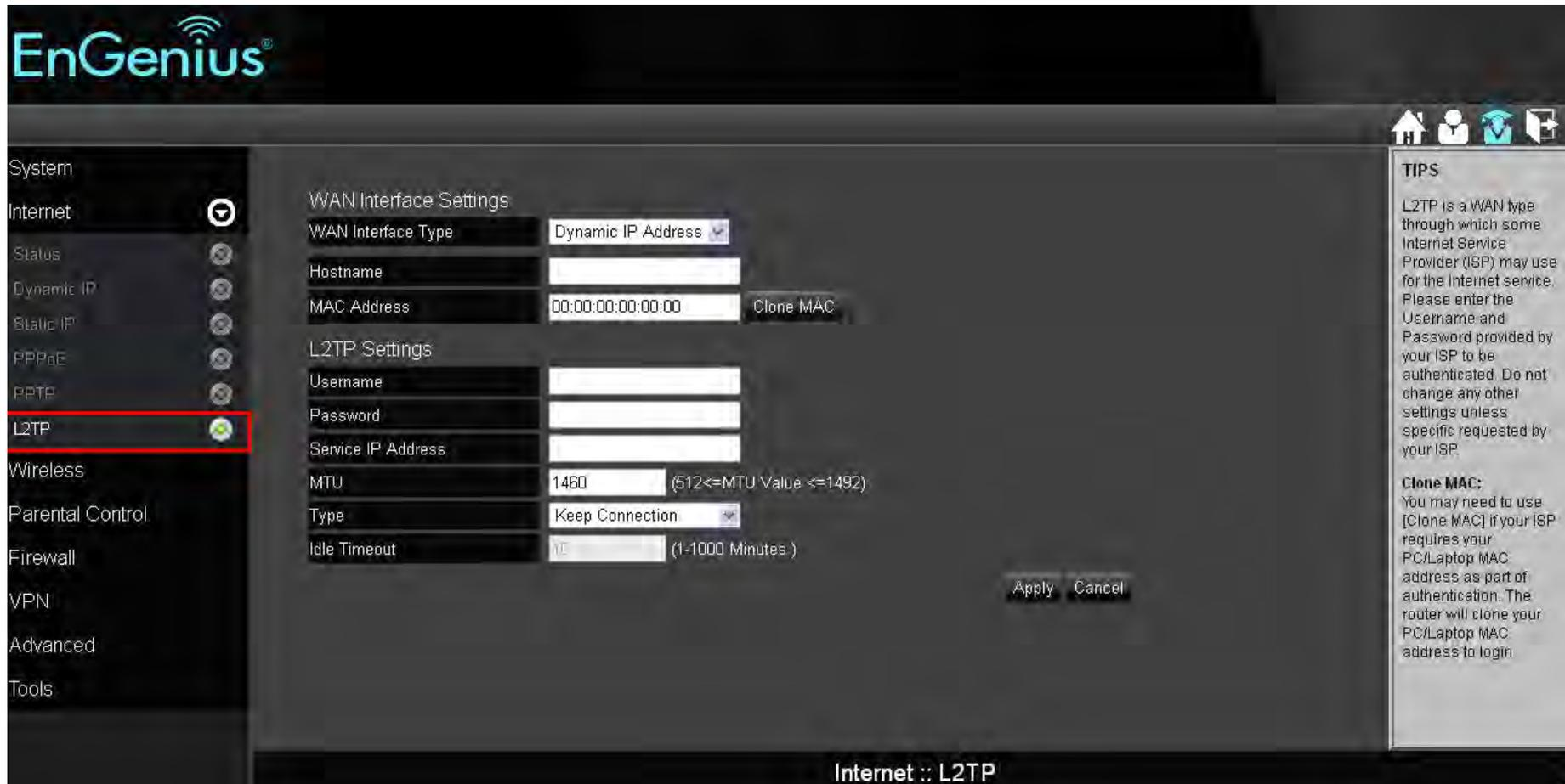
The screenshot displays the EnGenius router's web management interface. The left sidebar contains a menu with the following items: System, Internet (selected), Status, Dynamic IP, Static IP, PPPoE, PPTP, L2TP (highlighted with a red box), Wireless, Parental Control, Firewall, VPN, Advanced, and Tools. The main content area is titled "WAN Interface Settings" and includes the following fields:
