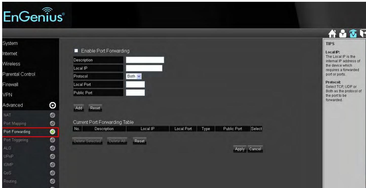
The screenshot displays the EnGenius web interface for configuring Port Forwarding. The left sidebar shows the navigation menu with 'Port Forwarding' highlighted in red. The main content area features a configuration form with the following fields:
