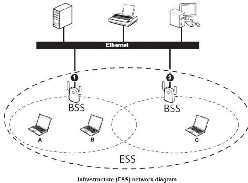
In an ESS environment, users are able to move from one access point to another without losing the connection. In the diagram below, when the user moves from BSS (1) to BSS (2) the WLAN client devices automatically switches to the channel used in BSS (2).
