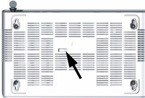
**Reboot function:** Press and hold the right end of the button for more than 1 second but less than 5 seconds to reboot the device. This does not affect the configuration settings.
