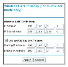
Figure 6-5: LAN IP Setup Menu
