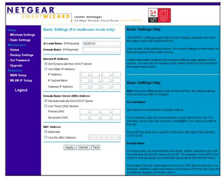
Figure 6-4: Switch position 2 login result: WGR101 basic settings page
