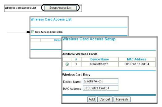
Figure 4-4: Wireless Card Access List Setup
