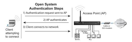
Figure D-1: 802.11 open system authentication
