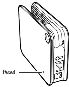
**Reset:** Press and hold the **Reset** key to restore the factory defaults.
