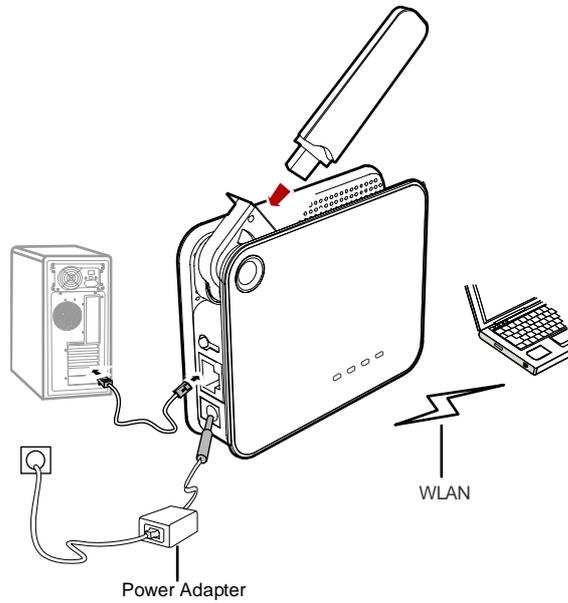
**Step 2: Connect to a PC through an Ethernet cable or WLAN.**
