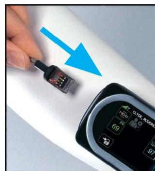
**Insert with connectors facing upwards**
