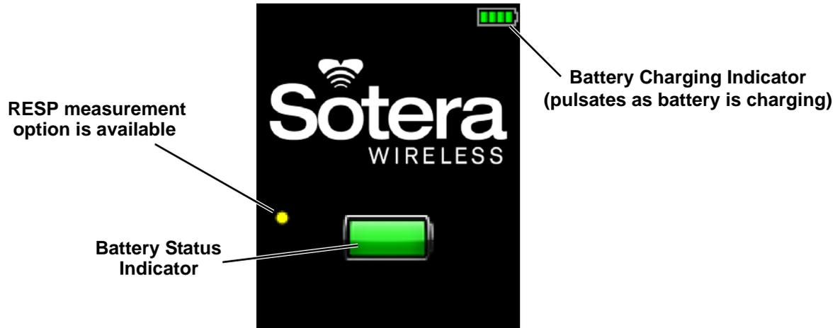
**Note:** When the yellow dot is displayed on the screen, it indicates the Monitor will measure RESP when a Chest Sensor is connected to a patient. RESP is not available as part of the default set of vital sign measurements and must be purchased separately.
