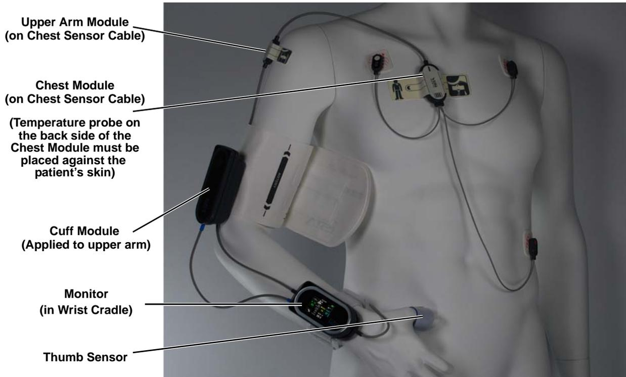
Whenever a sensor is connected to the Monitor, a self-test of that sensor is initiated automatically to verify the sensor is in good working order. If the sensor and Monitor speaker are in good working order, you will hear a double beep. This process takes a few seconds, after which monitoring of the selected vital sign commences as soon as the sensor is connected to the patient.
