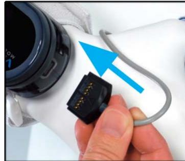
**Insert with connector contacts facing upwards**
