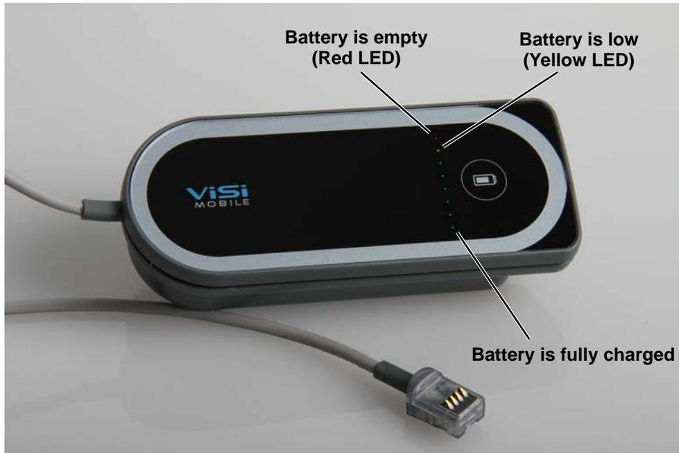
*When one of the green charging indicators is flashing, the battery in the Cuff Module is charging. The position of the green charging indicator represents the level of charge. When the charge indicator furthest away from the red charging indicator is flashing, the Cuff Module is fully charged.*
