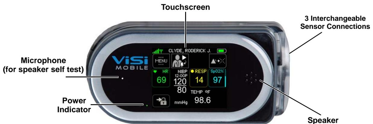
**Note:** The power indicator shows the level of Monitor's battery charge by flashing green (the battery has at least 2 hours of monitoring time left), yellow (the battery is low with less than 2 hours of monitoring time left), and red (the battery is critically low with less than 30 minutes of monitoring time left).
