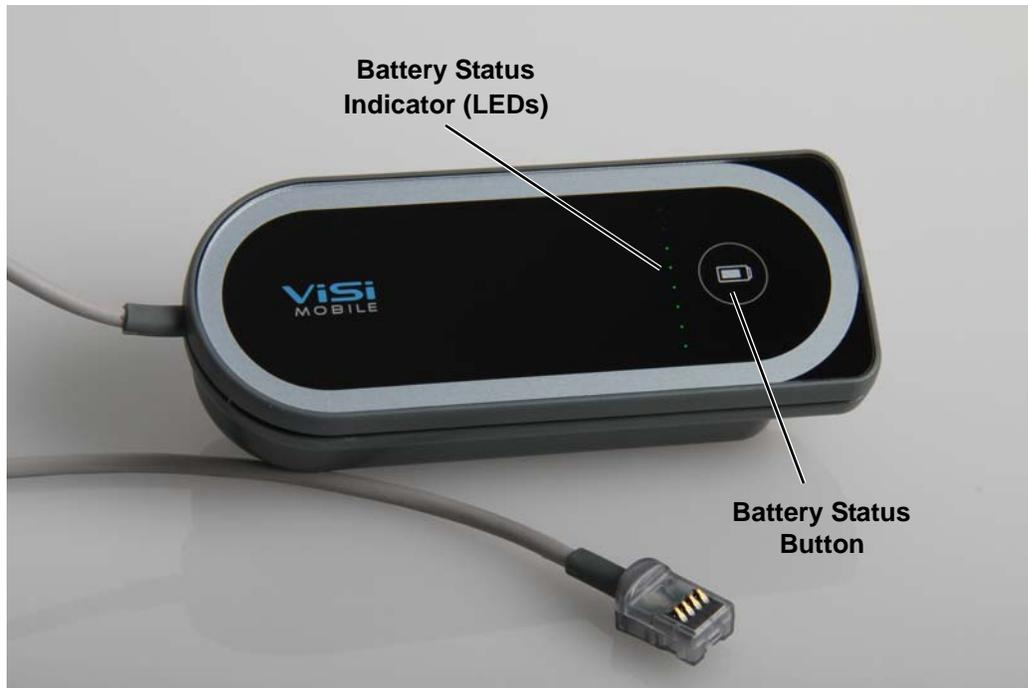
**Note:** When the battery status button is pressed, the battery status indicator shows the level of the Cuff Module's battery charge. Green lights indicate the battery has a minimum of 11% charge. More green lights indicate a greater charge level. A yellow light indicates the battery charge is less than 10%. A red light indicates there is less than 4% battery charge.
