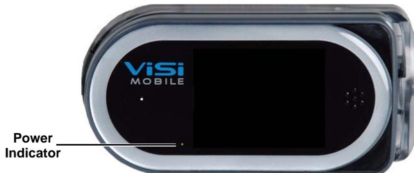
*The power indicator will blink while the Monitor is charging: green indicates there is enough charge to monitor a patient for at least two hours; yellow indicates the battery charge is low (less than two hours of monitoring); and red indicates the battery charge is critically low (less than 30 minutes of monitoring).*
