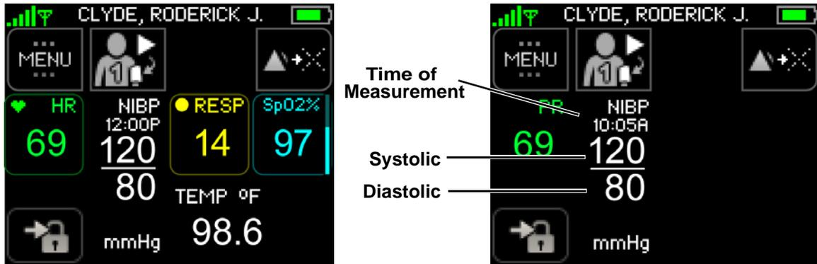
**Note:** If the NIBP measurement was unsuccessful, the Cuff Module automatically retries to measure the blood pressure. A maximum of 3 attempts will be made. If the failure is due to a cuff leak or cuff occlusion, there is no retry and the LEAK or OCCL message appears on the screen directly below the NIBP label.
