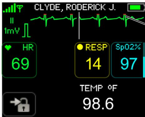
Positive limit of the dynamic range is being exceeded only at the peaks of the QRS complex of the ECG waveform
