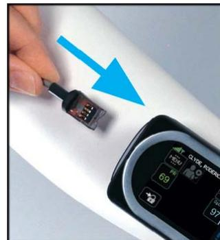
**Insert with connector contacts facing upwards**
