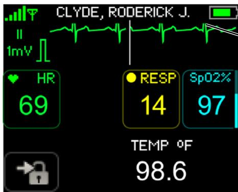
Dynamic range of the ECG amplifier has not been exceeded, but in which the peaks of the QRS complex of the ECG waveform extend beyond the upper edge of the display area
