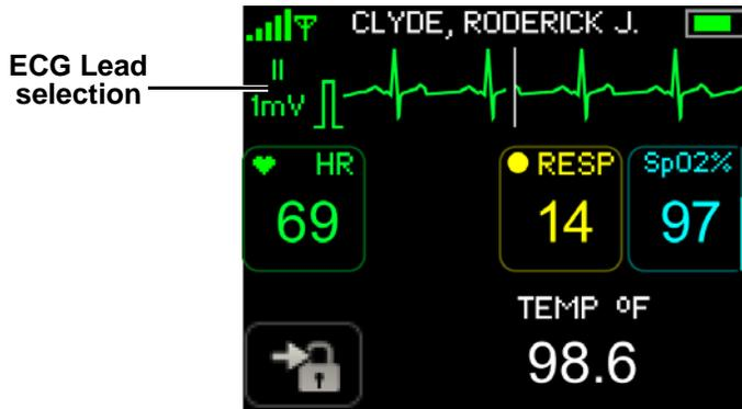
*The top third of the display is replaced with the ECG waveform. The displayed lead is indicated to the left of the waveform. The square wave indicates the standard calibration of the ECG waveform.*
