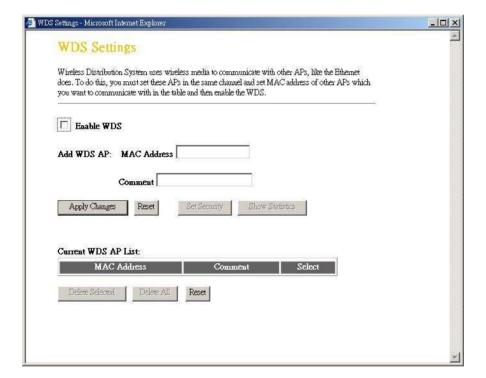
Wireless Distribution System allows this AP to communicate with other APs wirelessly. To make it work, you must ensure that these APs are in the same Channel and add these APs MAC Address and Comment values into the WDS list. Don't Forget to Enable the WDS by click the check box of "Enable WDS" and press "Apply Changes" button to save.
