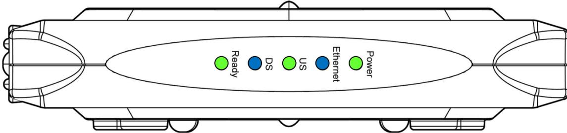
**Note:** The above LED pattern indicates Online Ready (Green), 2 to 4 Bonded Downstream Channels Being Used (Blue) for Increased Speed to the Internet/Cable Network, 1 Upstream Channel (Green), 1000Mbps Ethernet (Blue), and Power ON (Green).
