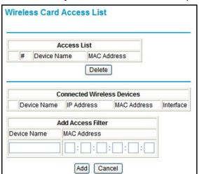
2. Click the **Setup Access List** button to display the Wireless Card Access List screen.
