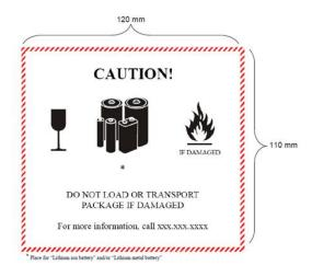
Label content for shipping smaller packages for batteries:
