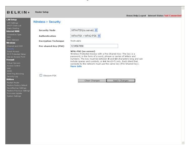
**IMPORTANT:** Make sure your wireless computers are updated to work with WPA2 and have the correct settings to get proper connection to the Router.
