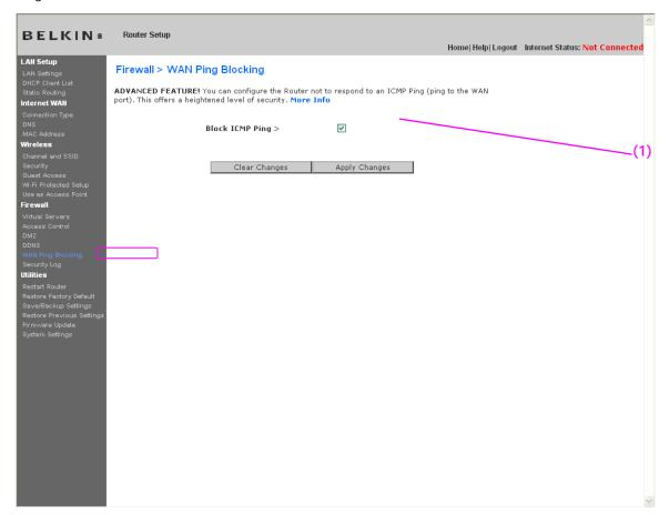
To turn off the ping response, select "Block ICMP Ping" (1) and click "Apply Changes". The Router will not respond to an ICMP ping.
