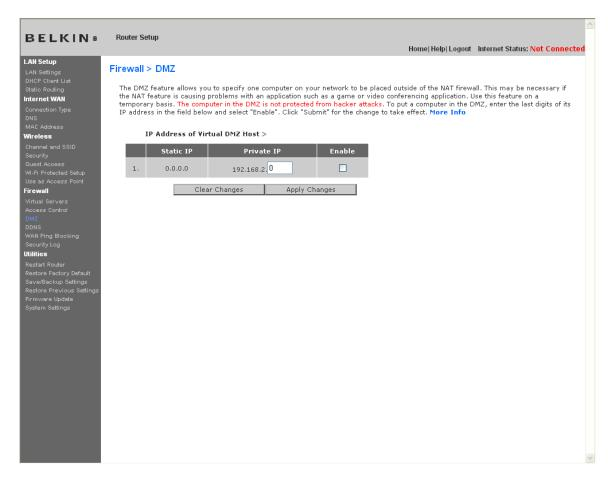
To put a computer in the DMZ, enter the last digits of its IP address in the IP field and select "Enable". Click "Apply Changes" for the change to take effect. If you are using multiple static WAN IP addresses, it is possible to select which WAN IP address the DMZ host will be directed to. Type in the WAN IP address you wish the DMZ host to direct to, enter the last two digits of the IP address of the DMZ host computer, select "Enable" and click "Apply Changes".
