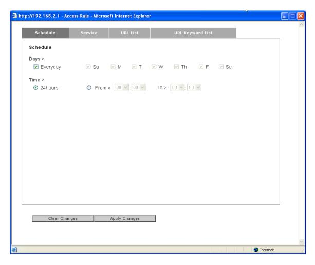
There are four main configurations for Access Control lists. The first one is "Schedule" for that rule. The second is "Service" for the services to be blocked for that rule. The third is "URL Blocking" for the URL access restrictions, and the fourth is "URL Keyword Blocking" for certain keywords to be blocked in the URL address.
