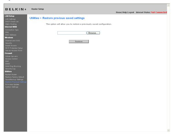
1. Click "Browse". A window will open that allows you to select the location of the configuration file. All configuration files end with a ".conf". Locate the configuration file you want to restore and double-click on it.
