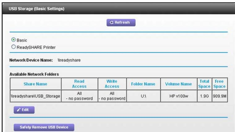
By default, the Basic radio button is selected, and the screen displays a USB storage device if it is attached to the router USB port.
