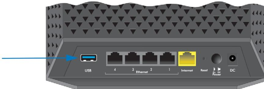
**Note:** Some USB printers (for example, HP and Lexmark printers) request that you do not connect the USB cable until the installation software prompts you.
