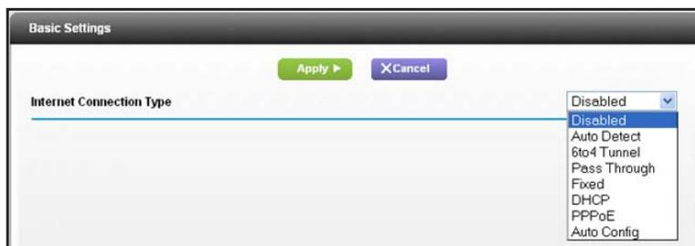
2. In the Internet Connection Type list, select the IPv6 connection type. Your Internet service provider (ISP) can provide this information.
