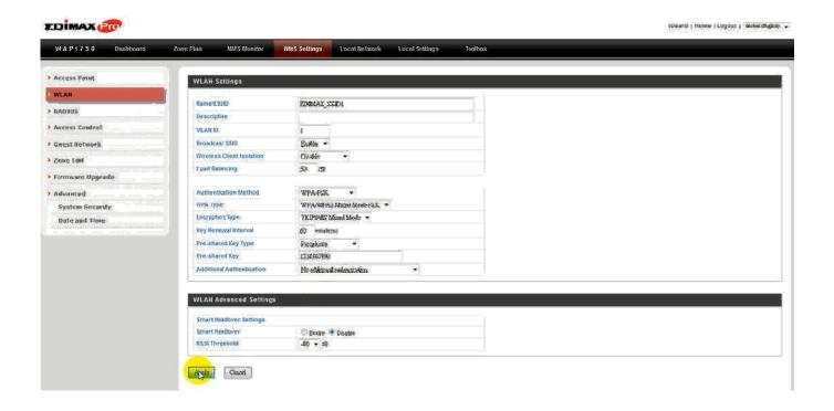
**3.** The new SSID will be displayed in the **WLAN** panel. **Repeat** to add additional SSIDs according to your preference, and then click "Add" in the **WLAN Group** panel:
