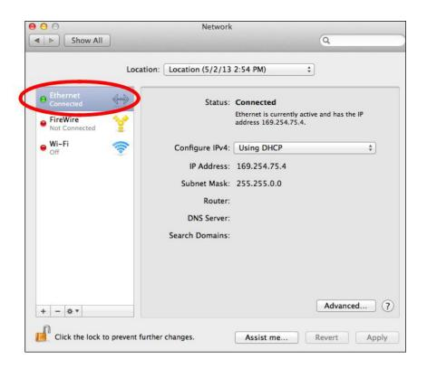
**4.** Open the drop-down menu labeled "Configure IPv4" and select "Manually".
