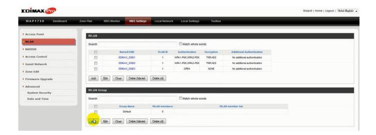
**4.** Enter a **name** for the **SSID group** and **check the boxes** to select which SSIDs to include within the group. Click "**Apply**" when done.
