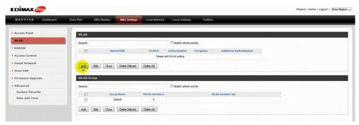
2. Enter an SSID name and set authentication/encryption and click "Apply":
