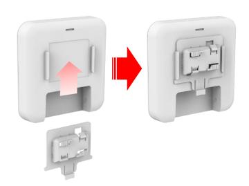
Select an appropriate ceiling mount base (9/16" or 15/16") and slide the base into the slot of the AP.
