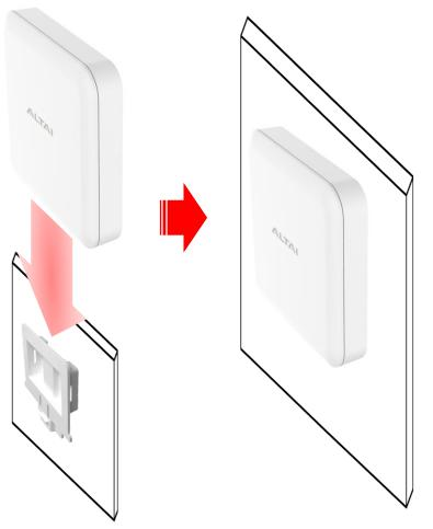
Slide the base into the slot of the AP.
