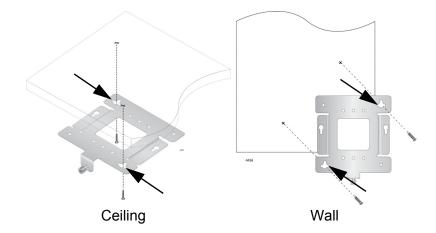
Figure 8. Marking/Pre-Drilling Holes the Mounting Bracket Key-Holes
