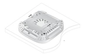
Figure 17. Seat Access Point onto Mounting Bracket
