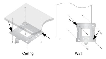
Figure 10. Pre-Drilling Holes on Mounting Bracket
