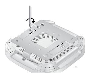
Figure 6. Adjusting the Screws on the Access Point
