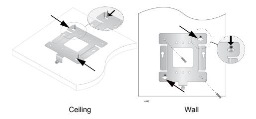
Figure 9. Mount Bracket On Screws Using Key-Hole Slots
