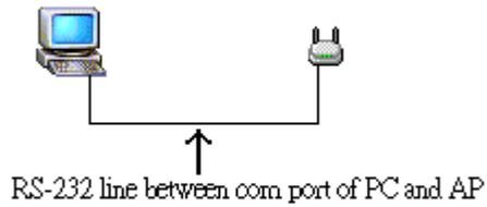
The basic setting of the terminal program is baud rate: 38400 bps, 8-N-1, no flow control. Please refer to the following graph.
