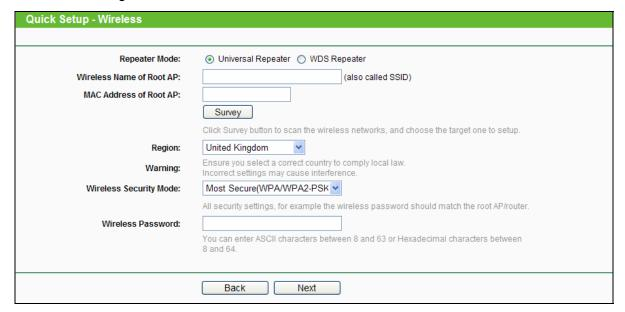
Figure 3-5 Wireless Settings – Repeater (Range Extender) mode
