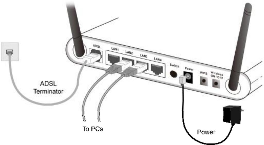
**Figure 4: Installation Diagram**
