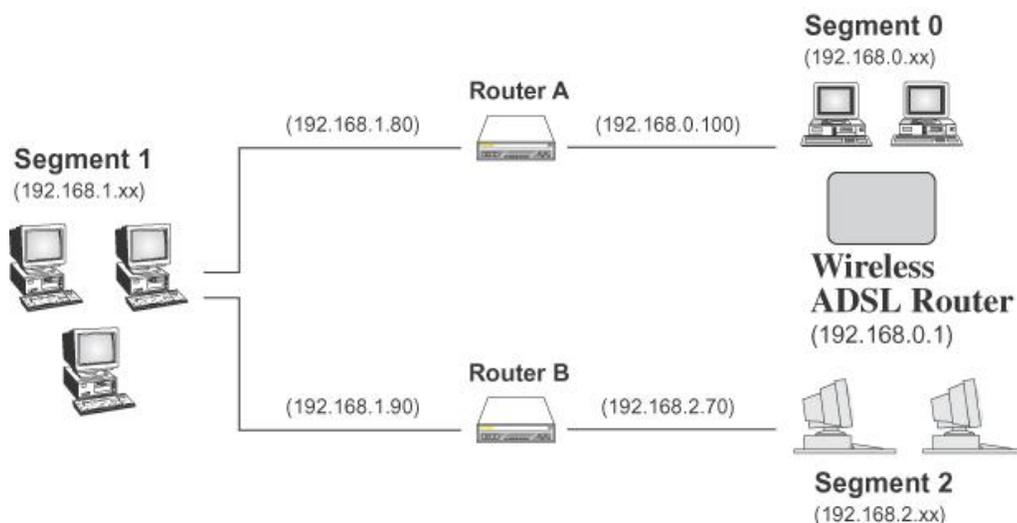
Figure 67: Routing Example
