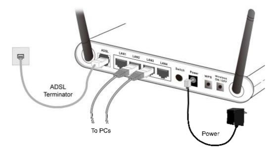
Figure 4: Installation Diagram
