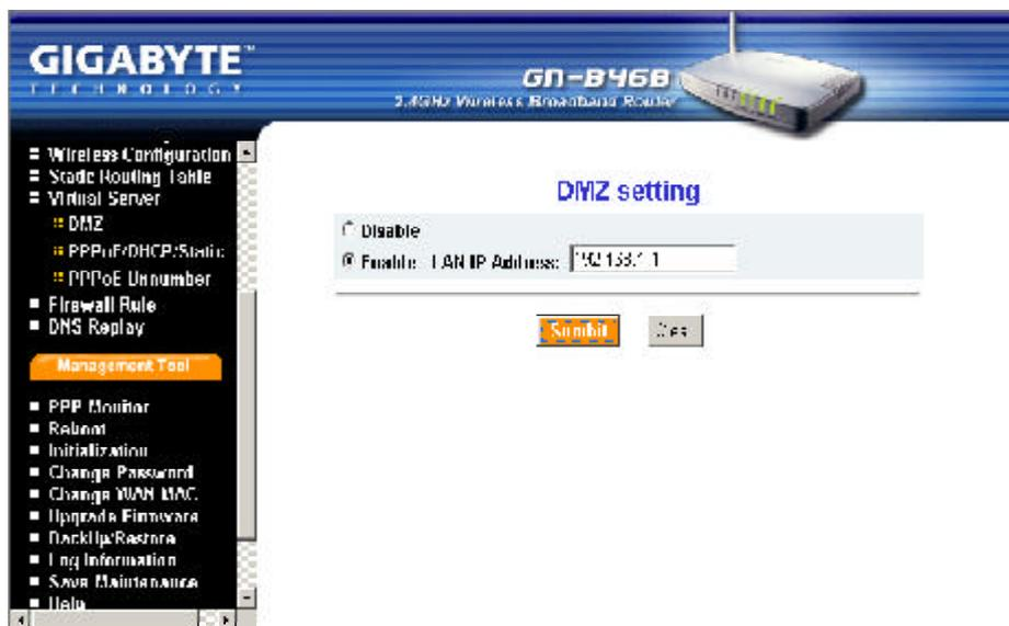
If you have a computer that cannot run an Internet application (e.g. internet game, video conferencing, or VPN connections) properly from behind the NAT firewall, then you can open the computer up to unrestricted two-way Internet access. To use the DMZ, you have to set a static IP address for the computer. The IP Address (such as 192.168.1.1) of the computer at the LAN terminal can be used to input to the field of LAN IP Address.
