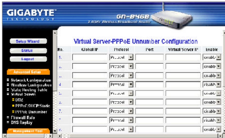
The PPPoE Unnumber user may have multiple global IP addresses, therefore each IP address needs to setup specifically.
