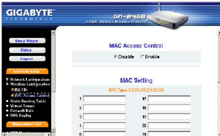
The MAC Access Control allows the router to define up to 32 hosts which are allowed to access to the WAN port. To disable the MAC Access Control function, keep the default value, **Disable**. To set up a MAC setting, click **Enable**.
