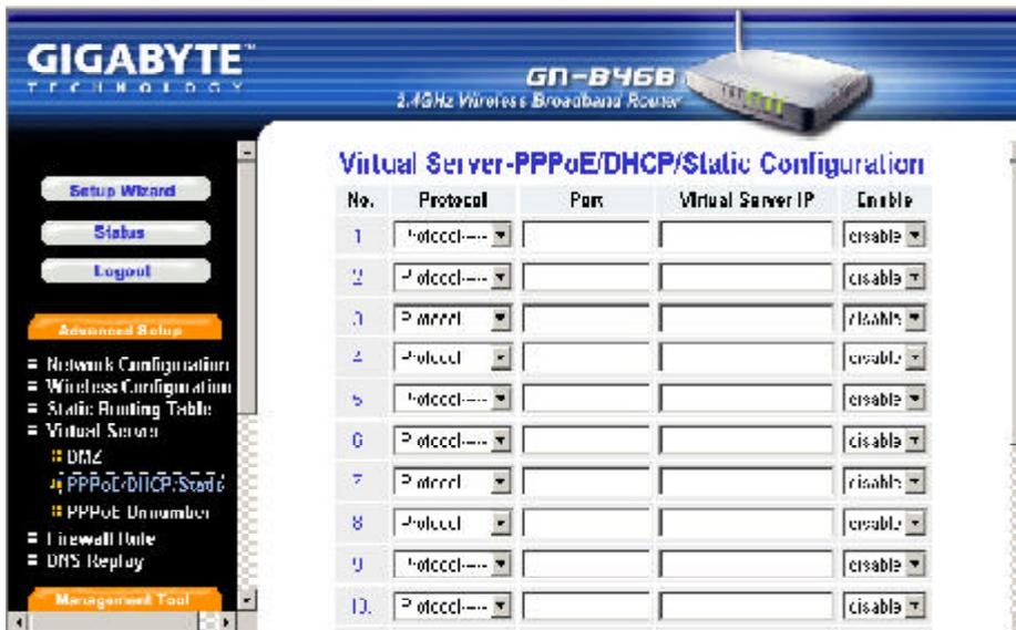
Virtual Server provides a way to let the PC at the WAN end connect to a server of a PC at the LAN end. Taking the IP address 192.168.1.1 of a PC on a FTP at the LAN for example:
