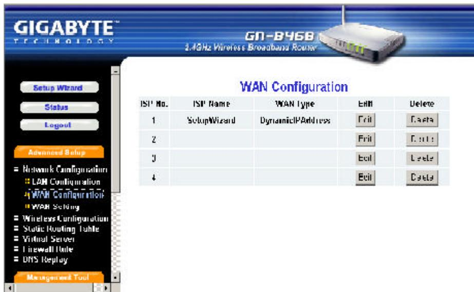
This page is the further configuration of the WAN connection. You can setup up to 4 WAN connection entries. Each entry may has it's own connection type (PPPoE, PPPoE Unnumber, Dynamic IP address, Static IP address) and some other properties. For example, when you click the “**Edit**” button of the ISP No.1 (WAN Type: Dynamic IP Address) on the table then there will appear the screen as follows.
