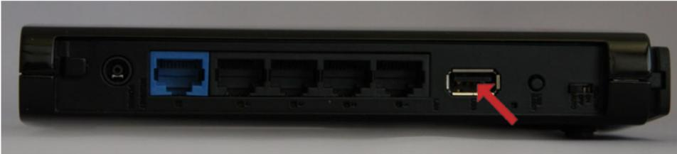
To add a USB hard drive or memory stick to the AirStation, plug it in to the AirStation's USB port.
