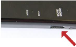
The AirStation may be configured to optimize data transfers according to either of two QoS models. The switch has two positions:
