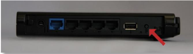
To release the USB device, hold down the USB Release button for 3 seconds. The USB device will be dismantled. When the USB LED stops blinking, it is safe to unplug the USB drive.
