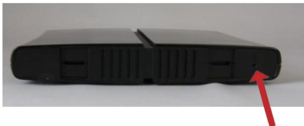
You may also initialize your AirStation by holding down the *Reset* button on the bottom for 3 seconds with a straightened-out paper-clip or similar object.
