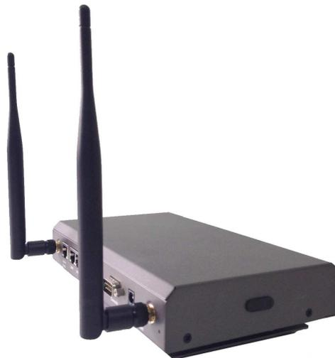
There is a hole on the right side for Kensington lock. If it is not used, admin can fill the hole with the rubber plug given.
