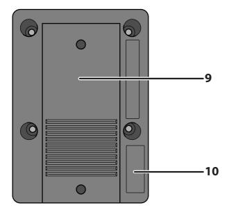
**9 Wall Mount Plate** Slide this plate out to wall mount. Attach to the wall with the 2 screws (included). Then, slide the AirStation onto the plate.
