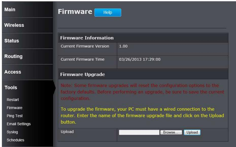
**Upload:** Click the **Browse** button to navigate to the new firmware file located on the management computers, and click the **Upload** button to initiate the firmware upgrade procedure. The firmware upgrades sometimes will reset the configuration to the factory defaults. Make sure to save the current configuration to the management computer, before performing firmware upgrade.
