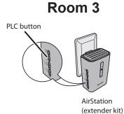
Within 2 minutes, hold down the PLC button of the AirStation that was installed in step 1 until the Power LED starts blinking green (about one second).
