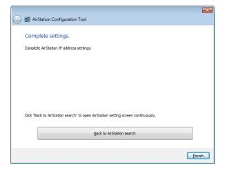
The new IP address is set to the AirStation. Once the settings are complete, the "Complete settings" screen is displayed. Click [Finish].
