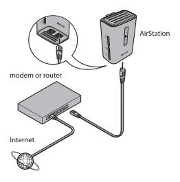
Connect one end of the LAN cable to the modem or router, and connect the other end to the Internet port of the AirStation.
