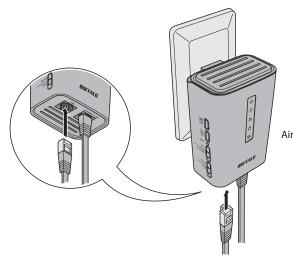
Connect the AirStation to your computer or TV. If using a wired connection, connect the AirStation LAN port to your computer or TV with a LAN cable.
