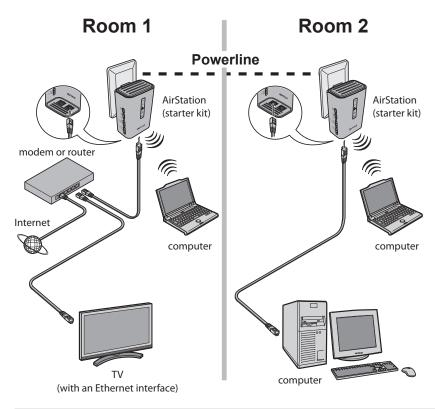
1 Check that connection to the Internet is possible without using the AirStation. Then, turn off the modem or router.
