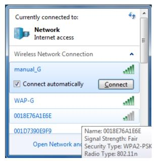
Select the target AirStation and click [Connect]. If you will be connecting to this device in the future, checking [Connect automatically] is recommended.
