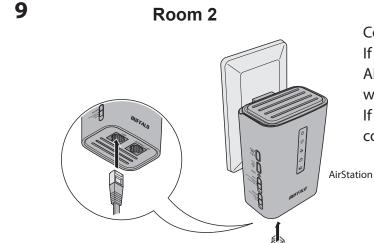
Connect the AirStation to your computer or TV. If using a wired connection, connect the AirStation LAN port to your computer or TV with a LAN cable.
