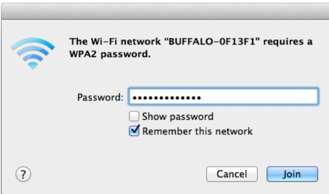
Enter the KEY from step 1 into the Password entry box, check [Remember this network], and click [OK].
