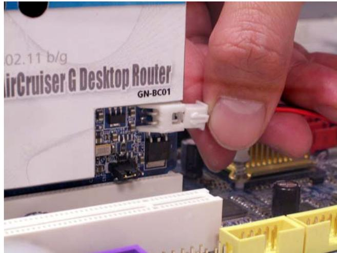
Figure 2-4 – Attach AirCruiser G power connector
