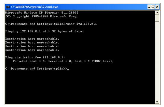
Figure 3-2 Failure result of Ping command
