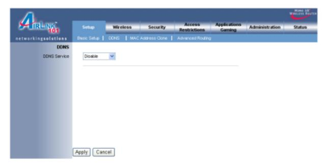
To Enable DDNS, select the DDNS provider you have registered with and enter the required fields. Click **Apply** to save the setting.
