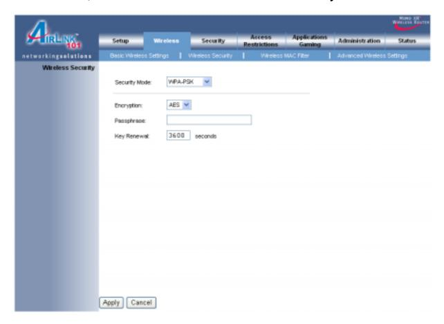
**Encryption**: Select either **TKIP** or **AES** as the encryption method.
