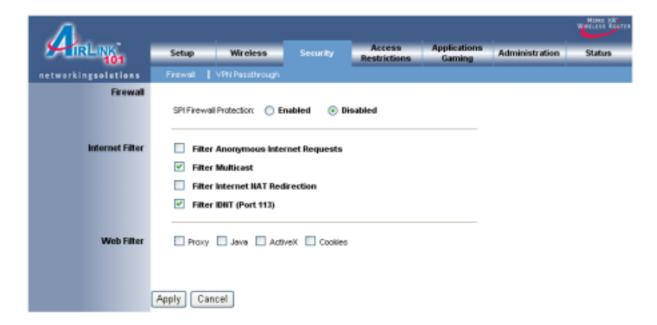
**SPI Firewall Protection**: Select to enable or disable Stateful Packet Inspection.
