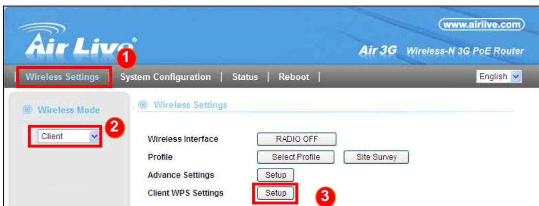
Select the SSID that you want to connect. Choose WPS mode to “Enrollee” and get a PIN Code in the field. Then press “PIN Start” and the “WPS” LED flash will light two minutes on the device’s housing.
