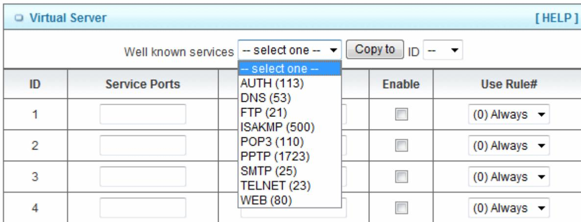
For example, if you have an FTP server (port 21) at 192.168.1.1, a Web server (port 80) at 192.168.1.2, and a PPTP VPN server at 192.168.1.6, then you need to specify the following virtual server mapping table:
