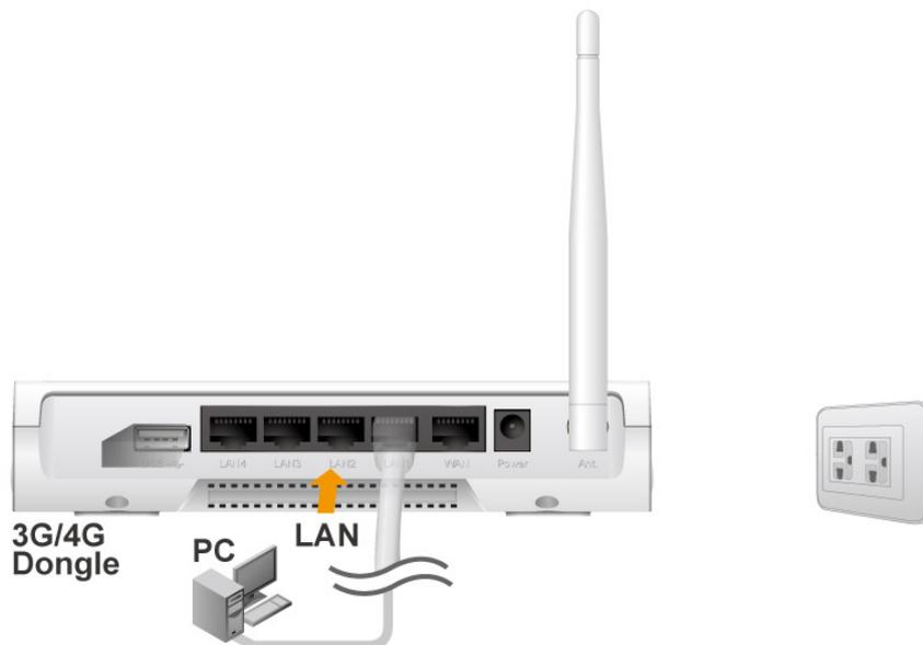
**Step 3.** Plug the power jack into the receptor on the back panel of the router. Then plug the other end into a wall outlet or power strip.
