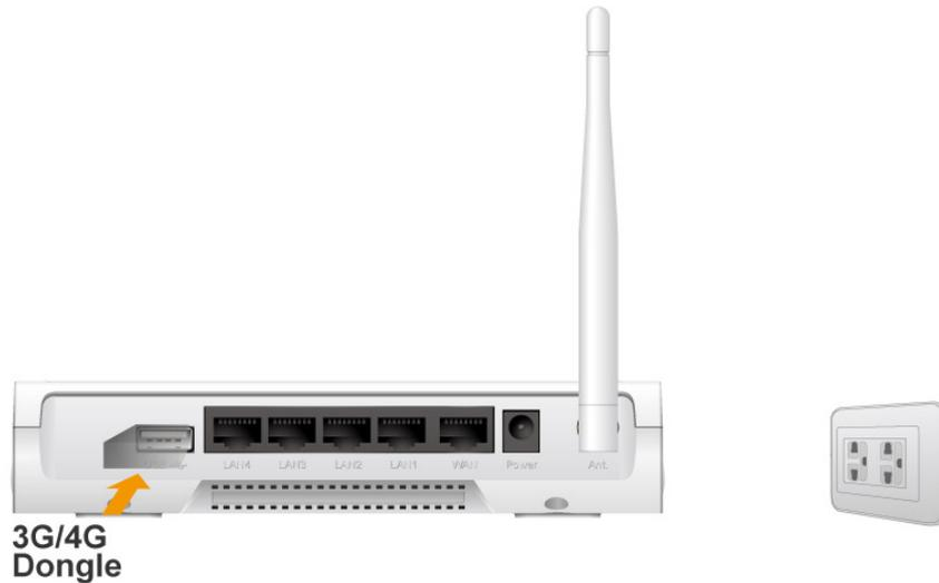
**Step 2.** Insert RJ45 cable into LAN Port on the back panel of the router. Then plug the other end of into computer.
