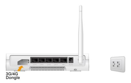
**Step 2.** Insert RJ45 cable into LAN Port on the back panel of the router. Then plug the other end of into computer.
